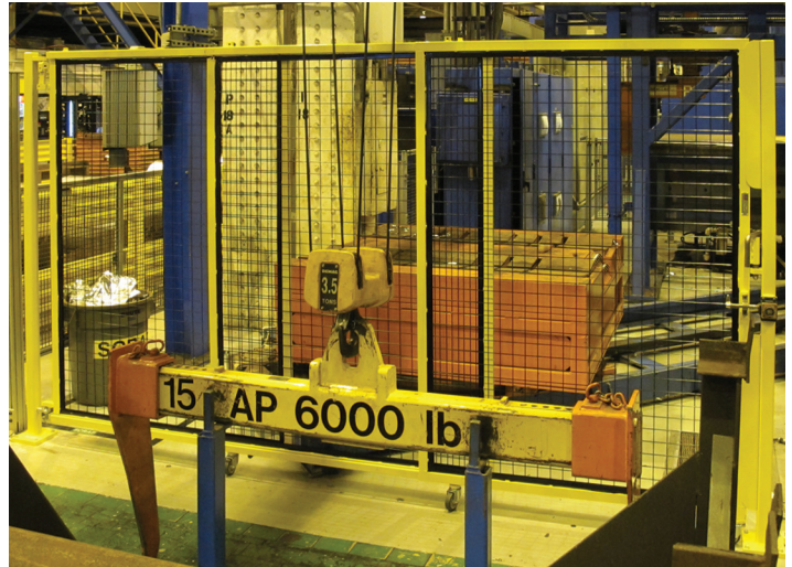
3-Panel Slide-A-Matic with black welded wire inserts. Note custom, factory installed interlock device.
